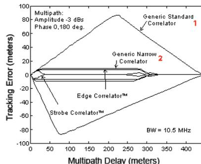
The horizontal axis of the plot shows the multipath delay, this is the extra distance that the reflected signal travels compared to the direct signal. The vertical axis shows the induced range error caused by a multipath signal with the indicated delay.
