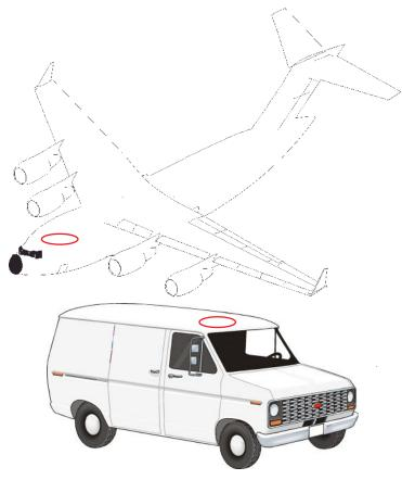
This graphic provides examples of where the antenna may be located on an aircraft or vehicle (not to scale).
