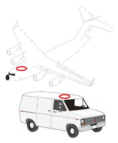
The graphic above shows examples of where the GPS-302-A antenna may be located on an aircraft or vehicle (not to scale).
