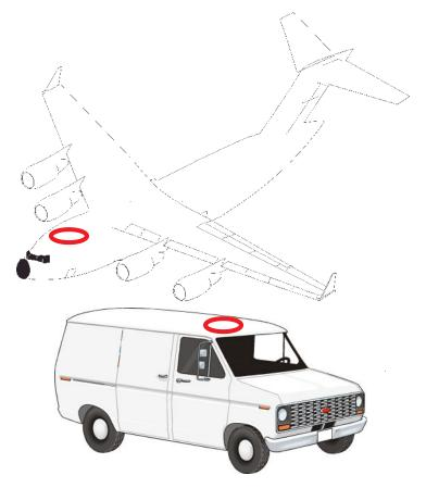
The graphic above shows examples of where the GPS-302L-A antenna may be located on an aircraft or vehicle (not to scale).
