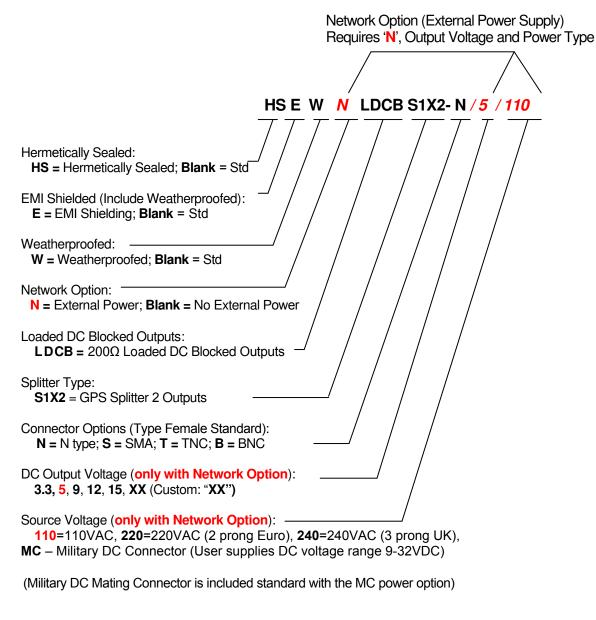
When no external power supply option (AC or DC) is selected, Output 1/J1 is Pass DC standard. Whenever an external power supply option is selected, all outputs are DC blocked standard.
