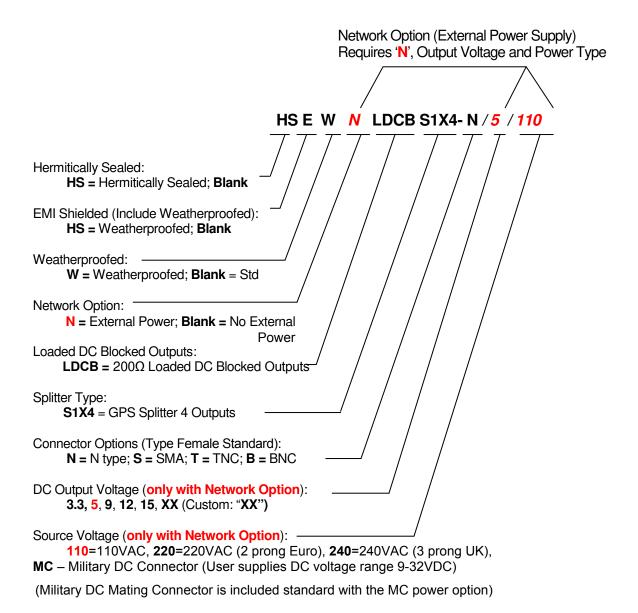
When no external power supply option (AC or DC) is selected, Output 1/J1 is Pass DC standard. Whenever an external power supply option is selected, all outputs are DC blocked standard.
