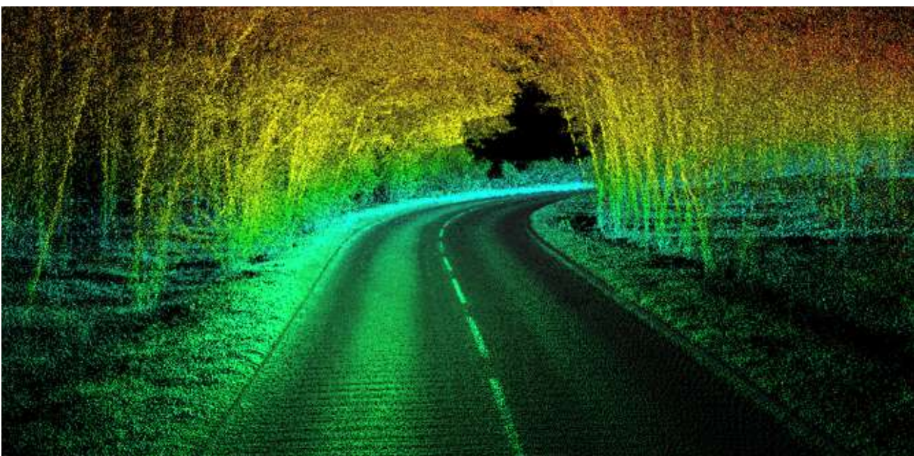
Road survey - pointcloud created using the Survey+ INS and Velodyne VLP-16 LiDAR sensor.
