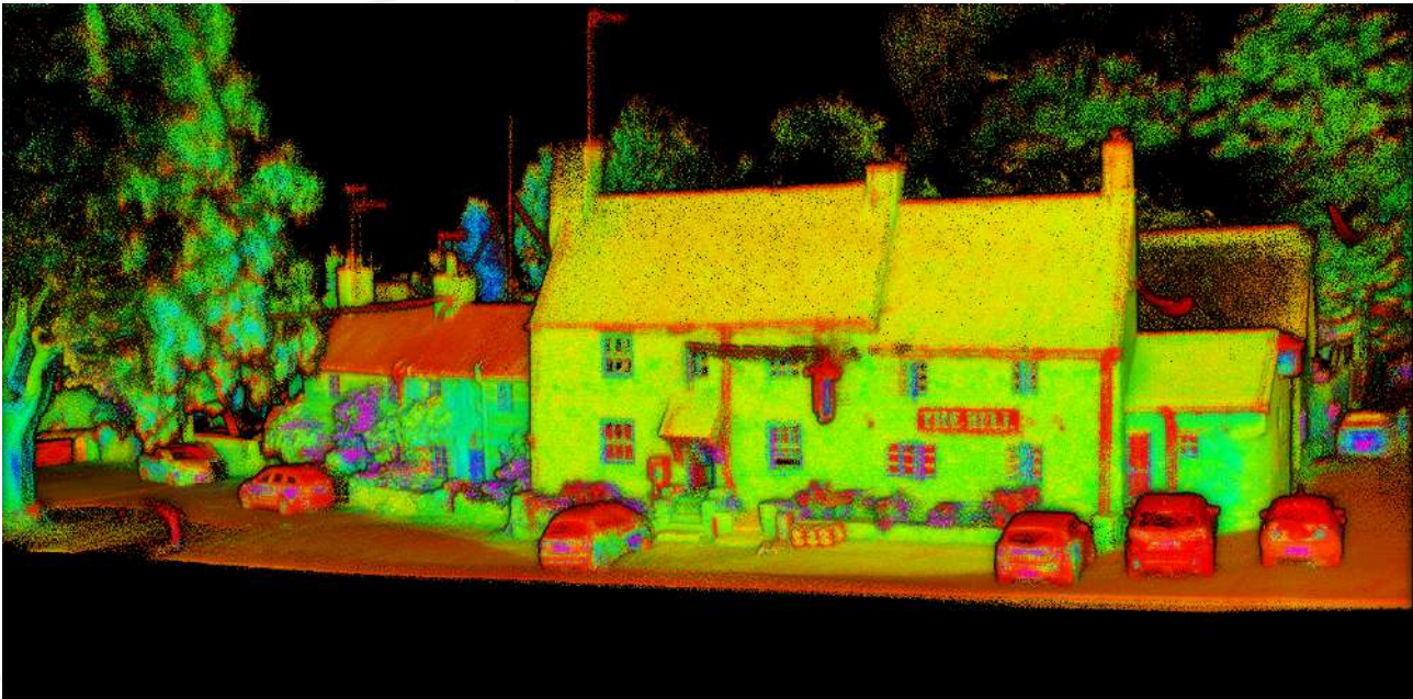
Building survey - pointcloud created using the xNAV650 INS and Livox Avia LiDAR sensor.
