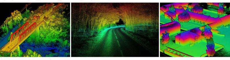
The pointclouds above were created by georeferencing the raw data from a LiDAR sensor with the inertial measurements from an OxTS INS. The bridge survey was conducted using a drone and the road and building survey data was collected on a mobile mapping vehicle (car).
