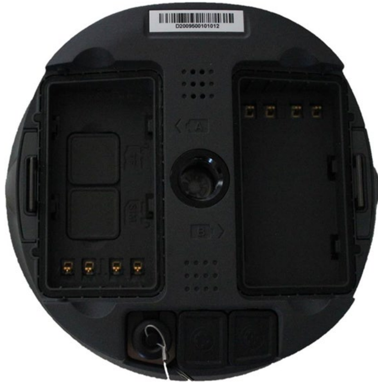
Figure 2-3: Battery compartment door removed
