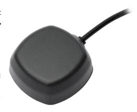
The TW4722 is the pre-filtered version of the TW1721. The pre-filter provides protection from near frequency or strong harmonic interfering signals. The TW4721/TW4722 is the smallest, lightest, wideband GNSS antenna available. It is housing in a compact IP67 magnetic or adhesive mount enclosure and is available with a wide range of connector options and custom coax cable lengths.
