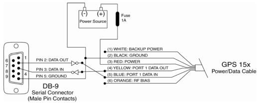
**Figure 2: PDA Serial Port Interconnection**
