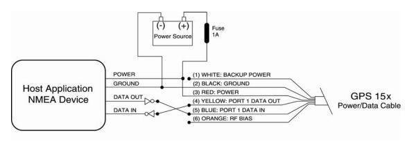
Figure 3: Basic NMEA 0183 Device Interconnection
