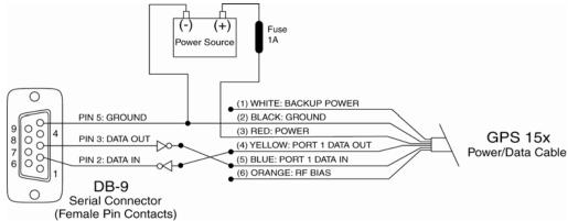
**Figure 1: Computer Serial Port Interconnection**
