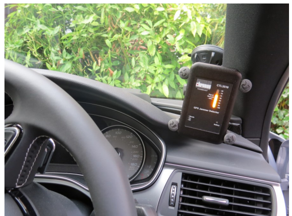
CTL3510 in cradle attached to windscreen
