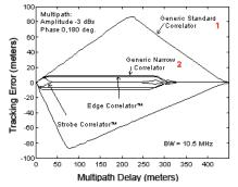
The horizontal axis of the plot show the multipth delay, this is the extra distance that the reflected signal travels compared to the direct signal. The vertical axis shows the induced range error caused by a multipath signal with the indicated delay.
