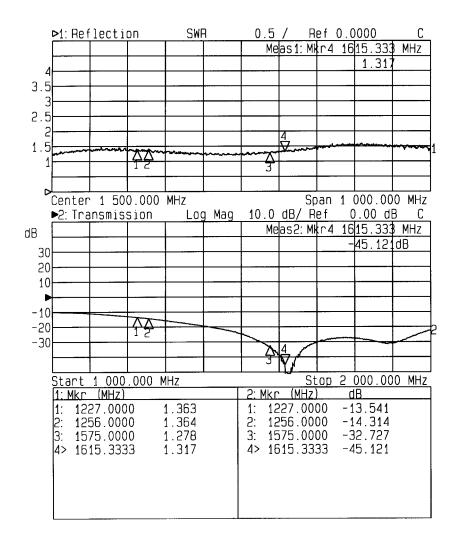
Output SWR (J1, J2, J3, J4) and Adjacent Output Isolation (J1-J3, J2-J4) (Typical, type N connector):
