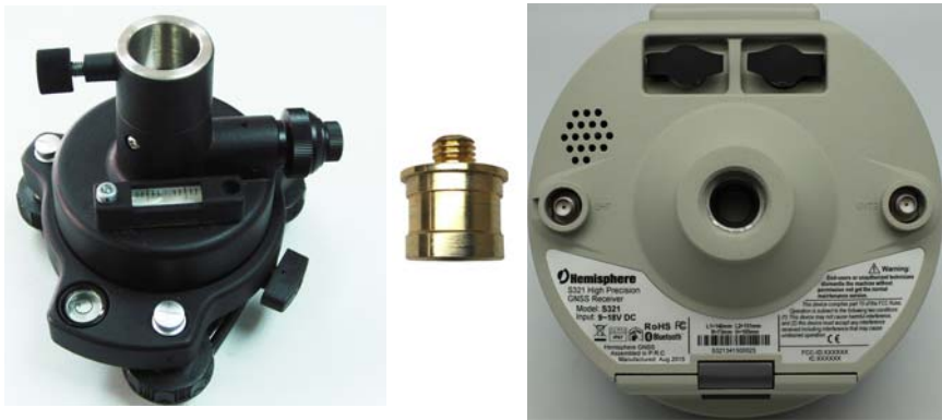
Figure 2-4: Installing S321 on a Tribrach
