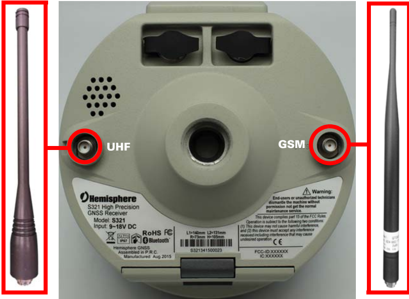
Figure 2-3: Installing UHF and GSM Antennas
