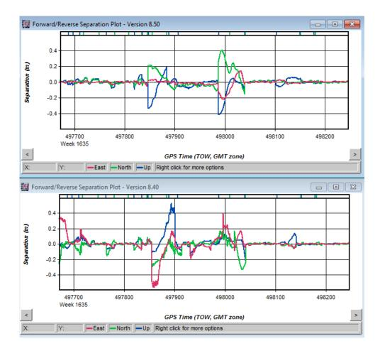
The new method also provides much faster recovery after a poor alignment. The above figures show an unsmoothed fwd/rev position separation plot for a ground vehicle survey after processed in both versions. The IMU used was a SPAN-FSAS IMU and the GNSS update rate was 10 Hz.
