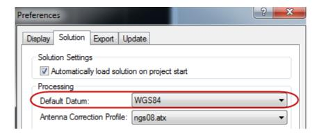
Previously, the datum could only be set when entering base station coordinates or, if processing PPP, through "Process GNSS" dialogue.
