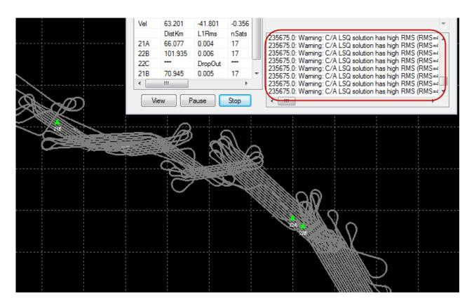
These warnings will not occur in version 8.50 as we now have a GPS/GLONASS time offset state for each base station in our filter, as opposed to one for the entire project.
