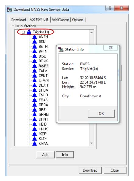
The FTP folder structure included the name of a city for each station in the 1s service above, which was not supported in version 8.40. We have added this field to 8.50 which makes it possible for us to support this service.
