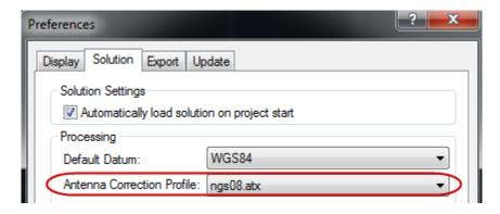
Inertial Explorer will perform relative to absolute antenna conversions internally if reprocessing projects created in previous versions. Therefore no special action needs to be taken by the user if reprocessing old projects.
