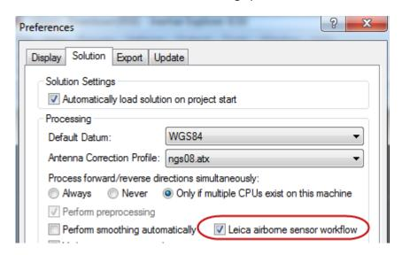
When enabled, raw Leica data (GNSS, IMU and gimbal) is converted to an Inertial Explorer readable format. A .sol file is also automatically produced after smoothing.
