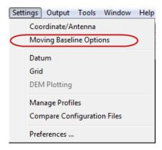
Only engage the moving baseline functionality if your base station is on a moving platform and you are interested in the relative vector between base and rover antenna. This is because in moving baseline processing the base station coordinates are not fixed. Thus, this mode of processing does not deliver accurate absolute positioning results.
