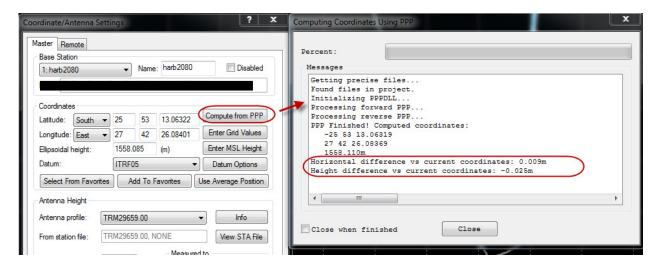
Using PPP for base station coordinate determination is a good choice if surveying in remote areas, far from other control points. This feature could also be used as a means to check loaded base station coordinates if several hours of data are collected.
