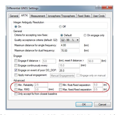
Every ARTK fix has an associated RMS and reliability. The RMS which indicates the level of agreement of the carrier phase measurements within the solution and the reliability indicates how much stronger the best solution is as compared to the second best. Having direct control over the maximum RMS and the minimum reliability is a powerful way of avoiding suspect fixes if poor fixes have been identified in the project.
