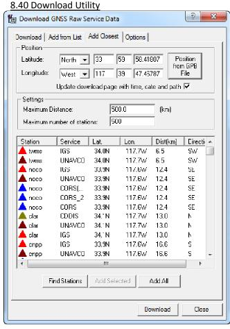
Further, version 8.40 no longer uses maximum distance and number of stations in its search. It will automatically apply a distance tolerance of 2,500 km and 2,500 stations, which should not be limiting for any application.
