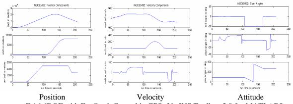
F-16 6DOF with Feedback Control in GPSoft's INS Toolbox 3.0 for MATLAB®
