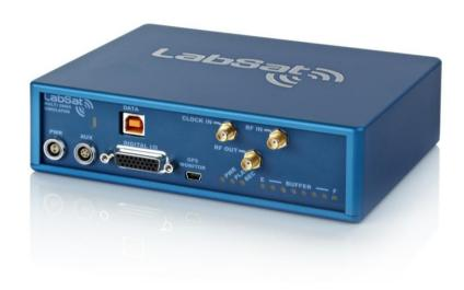
When replaying, the same data is streamed from the laptop to LabSat 2 at the same rate. A large internal buffer means that data is seamlessly replayed.
