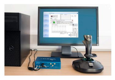
**LabSat RT** can play satellite signals from two constellations with a current time stamp. \*Joystick functionality will be available in a later version
