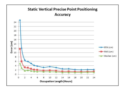
These graphs show the results of 36,000 processing runs using 1000 different CORS stations. GrafNav's SDK was used to automate all processing.
